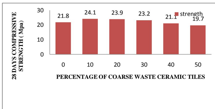
**Figure: 28-Days concrete compressive strength versus percentage of coarse waste ceramic tile in the mix**
