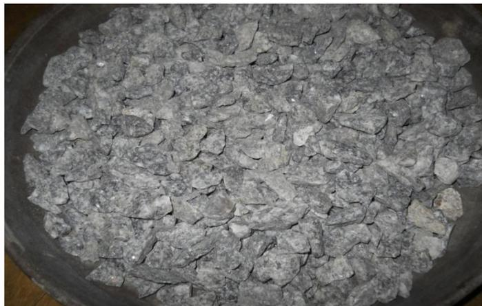
**Figure: Sample of the natural coarse aggregate for concrete mix**
