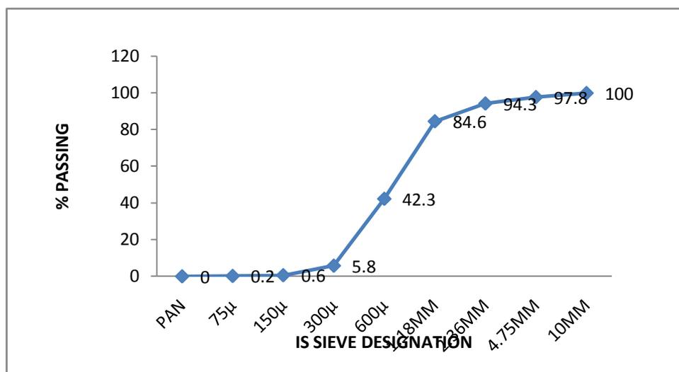
**Figure: Grain size distribution curve of fine aggregates**
