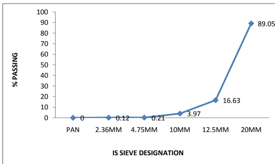
Figure: Grain size distribution curve of coarse aggregate
