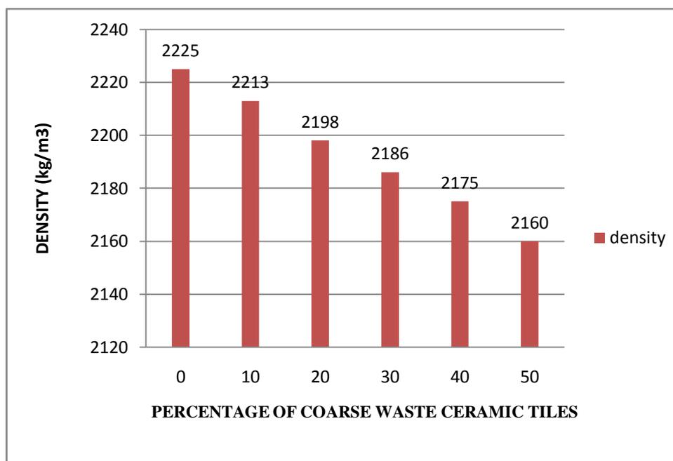
**Figure: concrete density versus percentage of waste ceramic tile aggregates**
