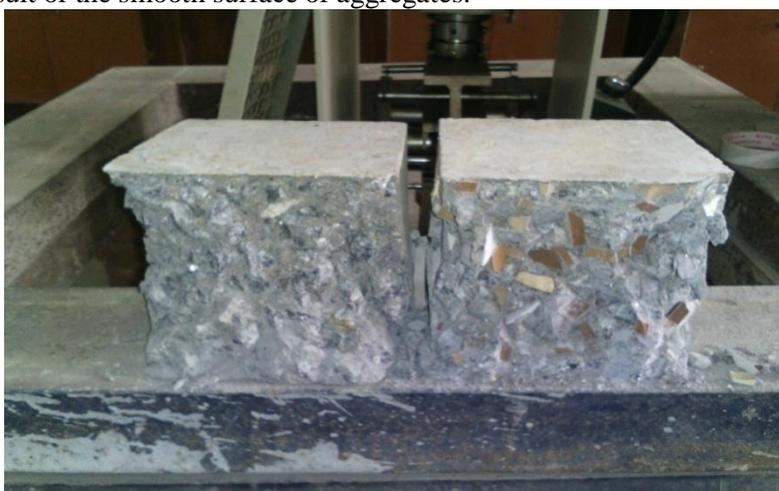
**Figure1: Typical testing reference cube (left) and waste ceramic tile cube (right) after failure for determining concrete compressive strength**
