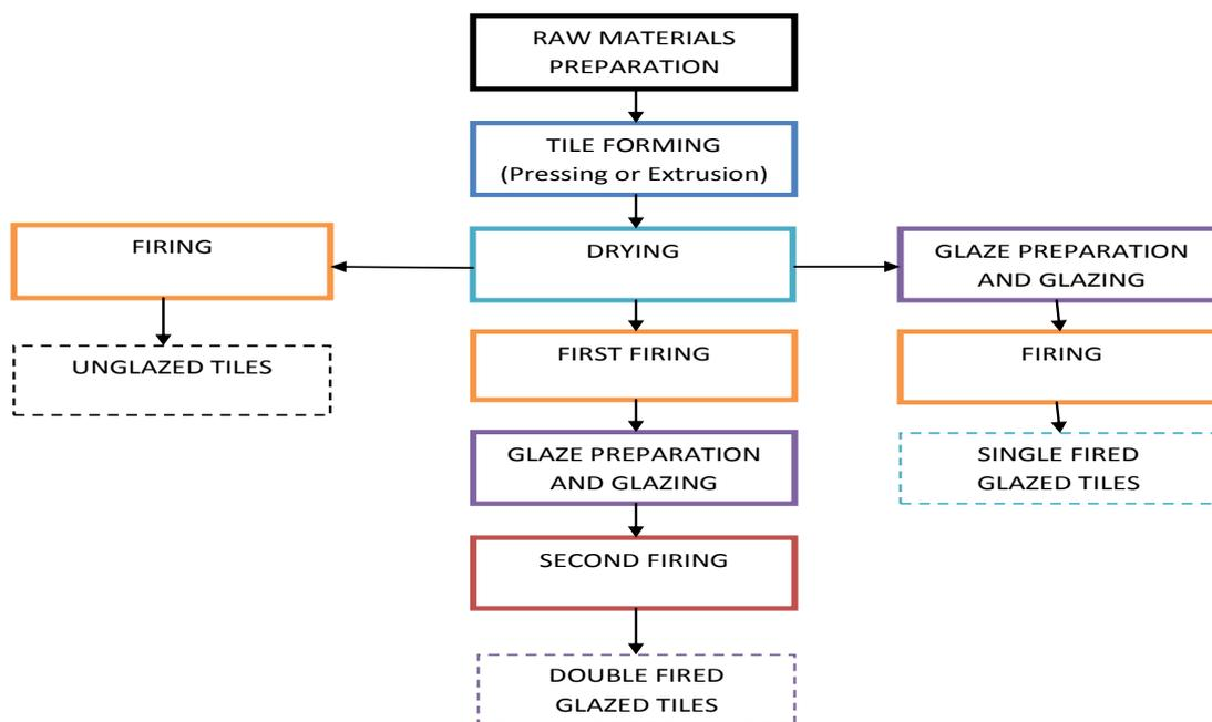
**Figure: Ceramic Tile Manufacturing Process**
