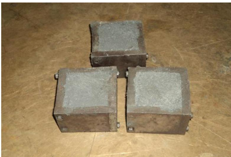
**Fig.: Cement Cube Specimens****TABLE: PROPERTIES OF CEMENT**
